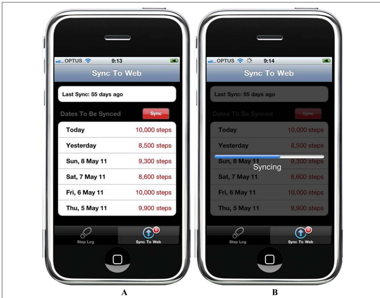
**Figure 2.** Sync to web screen changes: (A) premodification; (B) postmodification—addition of a progress bar to demonstrate to users that their request is being processed
