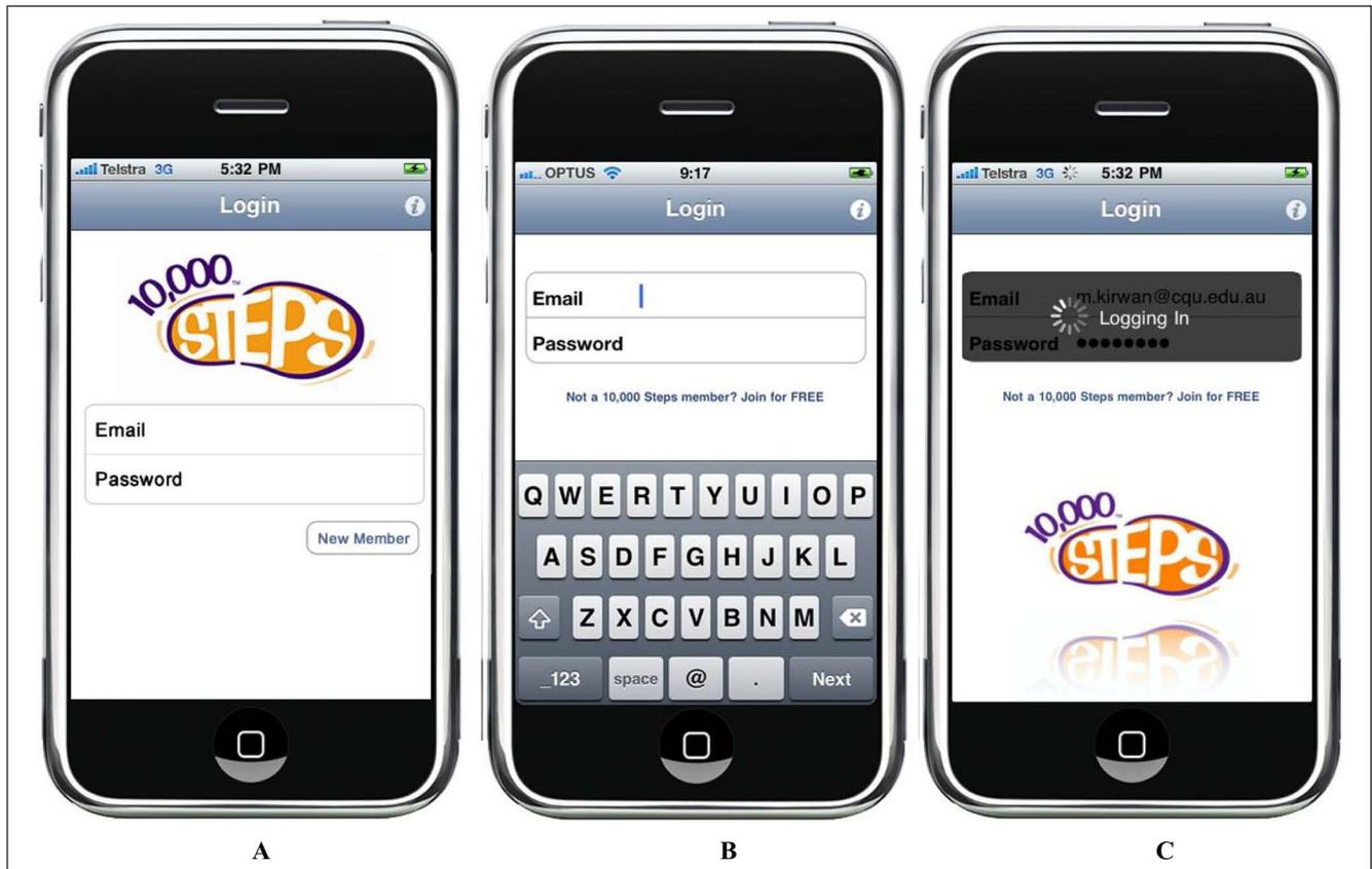
**Figure 1.** Login screen changes: (A) premodification screen; (B) postmodification screen—positioning of elements has changed, keyboard automatically appears, and cursor flashes to prompt user; (C) postmodification screen—a “logging in” icon communicates that the user’s request is being processed
